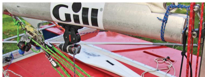
DOUBLE SWIVEL CLEAT WITH OUTHAUL AT THE REAR, AND LEECH CORD AT THE FRONT
