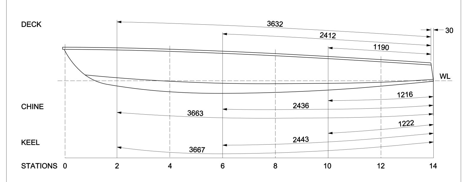
DIMENSIONS SHOWN ARE MEASURED FROM THE TRANSOM ALONG THE DECK CENTRELINE AND KEEL, AND AROUND THE CHINE. THESE POINTS PROVIDE A QUICK POSITIONING FOR THE HULL PROFILE MEASUREMENTS ON A STANDARD HULL.
